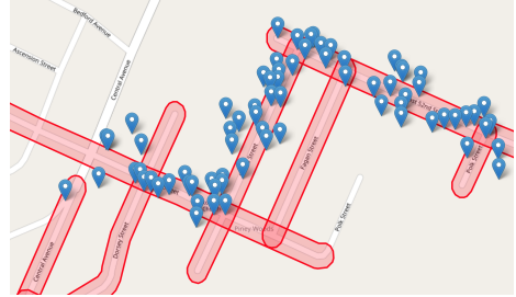
Fig. 4. Example of mapping locations to road segments without noise. Road segments that are output by Algorithm 1 are highlighted in red.
