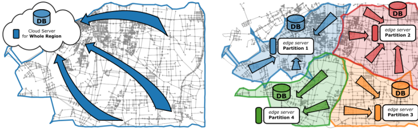
Fig. 4. Cloud-based Architecture (Left) vs Distributed/Edge-based Architecture (Right)
