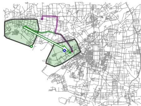
Fig. 8. Dest. Subroute Connection: Find and connect dest. subroute (green line) to basis route (purple line)
