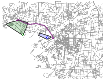
Fig. 9. Basis Route Merging: Merge routes and use as new basis route (purple line)
