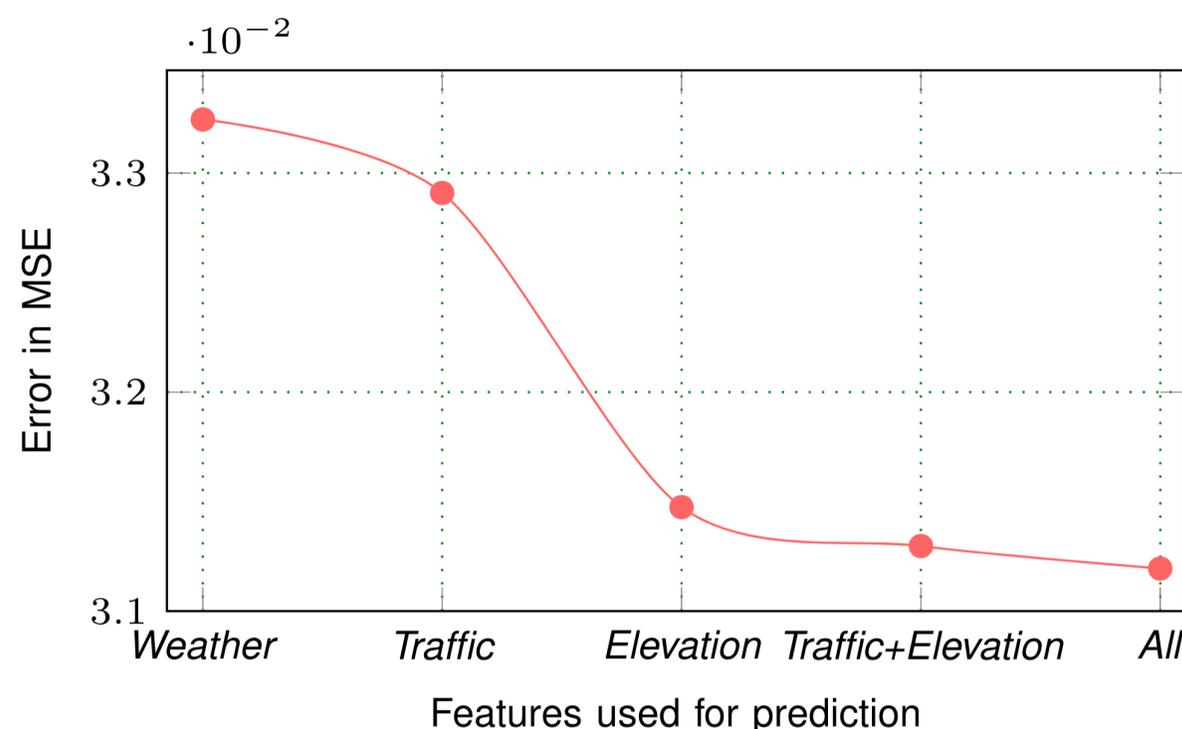
**Elevation is by far the most significant feature for electric vehicles**
