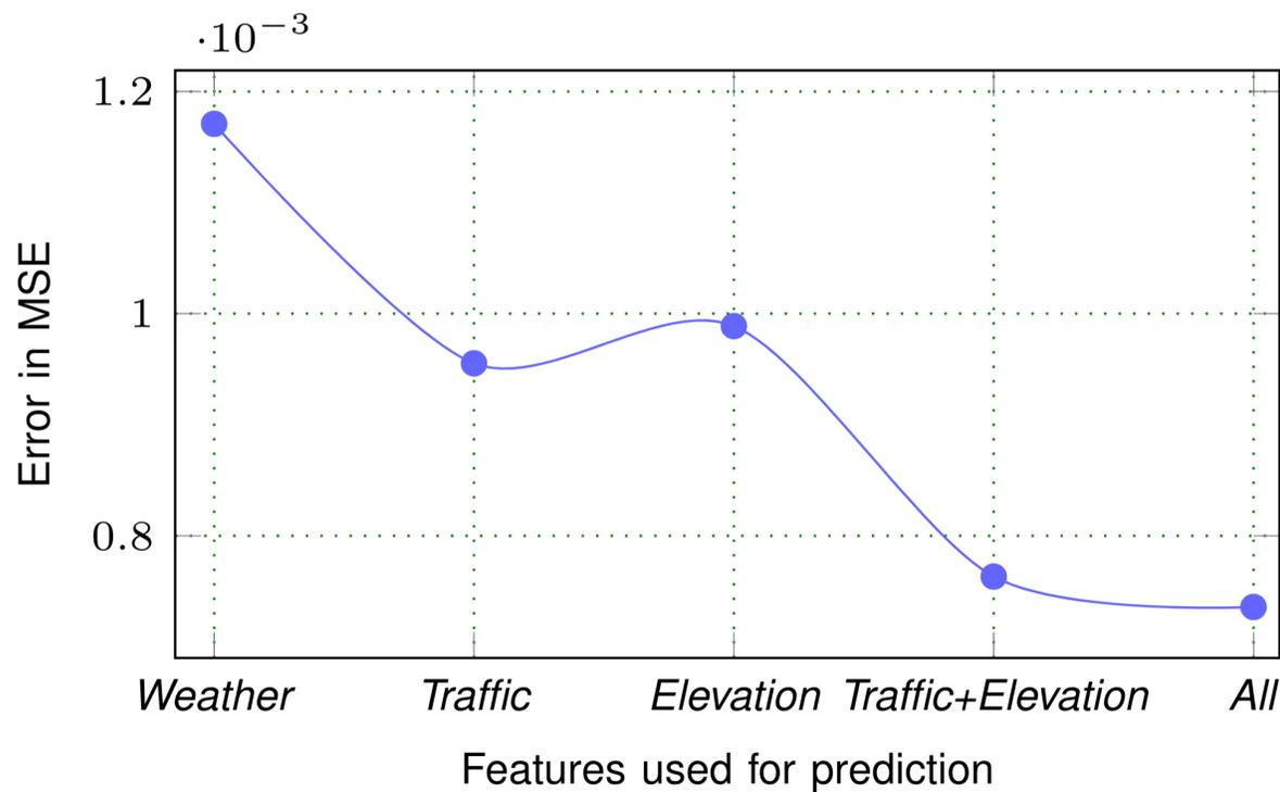
**Both elevation and traffic data are significant for Diesel vehicles**
