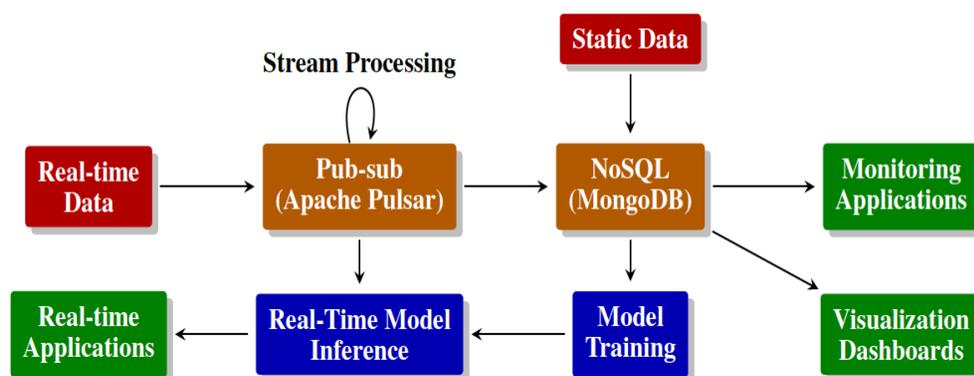
Data architecture overview - real time data is streamed to an Apache Pulsar cluster consisting of 5 broker/bookie nodes and 5 zookeeper nodes running on-site in VMWare. A MongoDB cluster running in Google Cloud reads from the Pulsar cluster, continuously updating its data view and adding spatial indexing for monitoring and dashboard applications.
