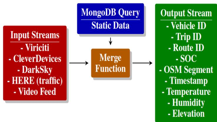
An example stream data join. Real-time telemetry and routing data from Clever Devices and ViriCiti are combined with weather from DarkSky, traffic from HERE and the video feed. The output stream includes all fields from these sources, as well as static data from OSM, GTFS and elevation. The output stream is updated periodically in real-time
